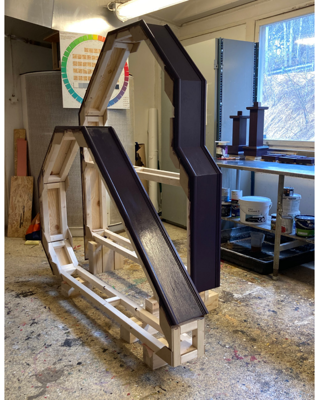
Figure 53-55: Plywood and wooden profiles attached, Ewing writing the glueing time, paint drying
