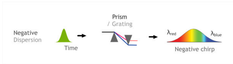
Figure 2.1: The effect of dispersion. Taken from APE (Angewandte Physik und Elektronik), "Dispersion Compensation and Pulse Compression" article.
