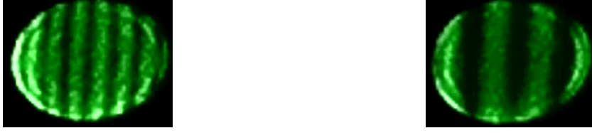
Figure 7: The number of interference stripes observed on the screen varies with the size of the droplet: larger droplets exhibit fewer stripes, while smaller droplets display a greater number of stripes. The average distance between the maxima is analyzed and utilized to determine the radius of the droplet.
