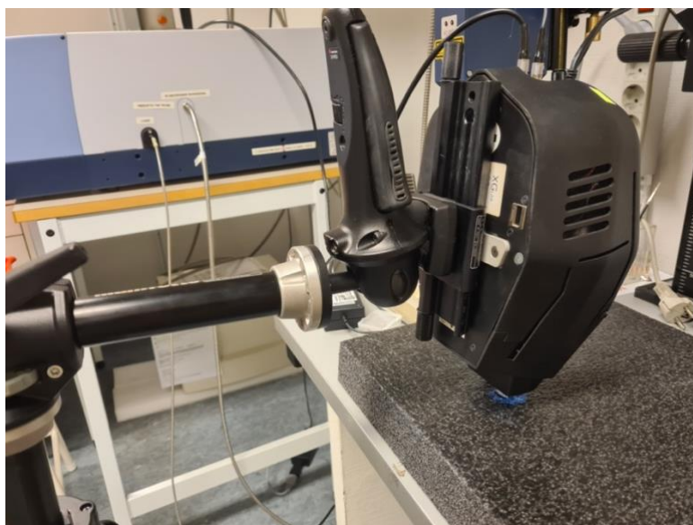
Figur 27. XRF under analys.
