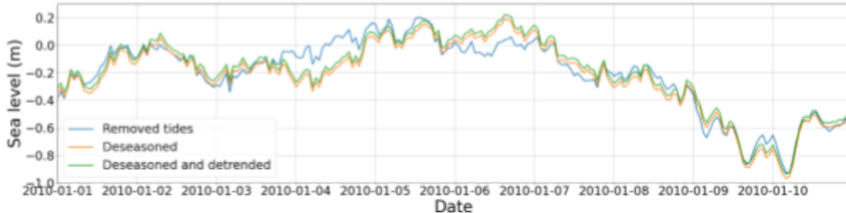
Figure 2.2 The data process of seasonal adjustment and detrending which results in the final data used in the model.
