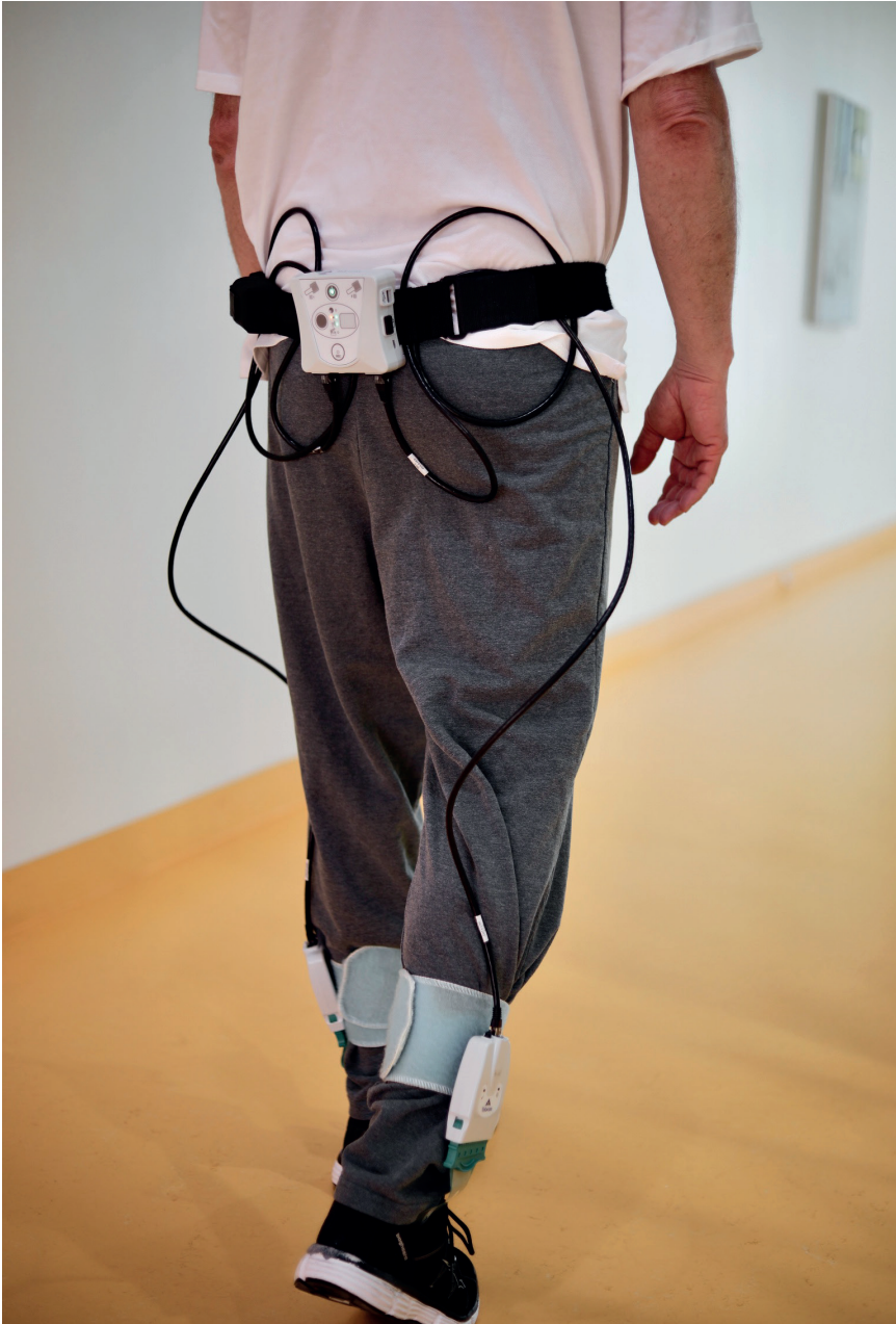
Figure 22. F-scan™ (Tekscan Boston, Massachusetts) wireless equipment. The sensors connected to a belt with a transmitter allowed the patient unrestricted walking within a certain radius.
