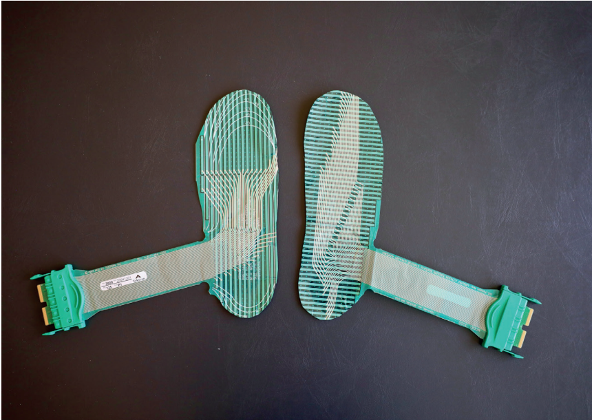
Figure 20. F-scan™ (Tekscan Boston, Massachusetts) sensor insole.
