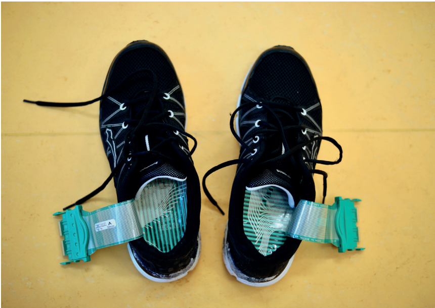
Figure 21. Shoes fitted with F-scan™ (Tekscan Boston, Massachusetts) sensor insole.
