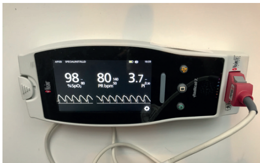
Figure 9: The perfusion index (PI) value is displayed at the very right, over the plethysmographic curve, and is in this example 3.7%. The oxygen saturation (SpO 2 ) is 98% and the heart rate is 80 beats per minute.
