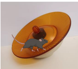
Figure 5. Med associates low-profile running wheel, used in ABA mouse model in conjunction with scheduled feeding for 2 hours per day.
