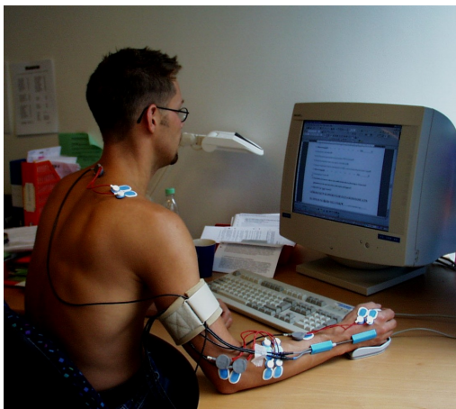
Figure 6. The position of the EMG electrodes.
