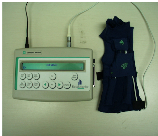
Figure 7. The instrument glove used to measure wrist positions and movements.
