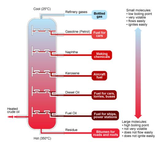
Note. The figure shows the distillation of crude oil to produce different types of fuel oils. Adapted from *Global Trading*, 2022. https://globaltrading.com/heavy-fuel-oil.php
