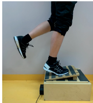
FIGURE 9: The heel-rise test was performed with a linear encoder attached to the heel while the patient performed single-leg heel rises with a 10° incline.
