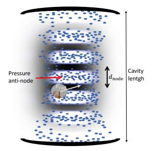
**Figure 3.7:** Acoustic pressure force  $F_{rad}$  (white arrow) on a small object immersed in the acoustic field balances the gravitational force  $F_g$  (brown arrow). Blue dots symbolize air particles. Anti-nodes are represented in the back by white regions, and in the front by high pressure (many particles). Nodes are represented in the back by black regions and few particles (low pressure)
