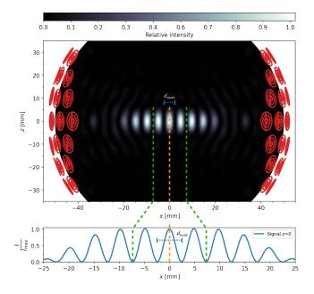
Figure 3. Simulation of acoustic trap. The black area shows the simulation of the acoustic field with relative intensity (grey scale) in the region accessible to the CCD. The structures in red color represent the positions and orientations of the transducers. The lower subfigure shows the relative intensity of the acoustic field along the x-axis for the central nodes of the trap.
