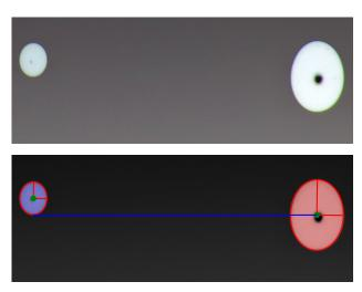
**Figure 4.9:** Upper: Image of two levitated droplets. Lower: Extracted pixel data from the upper image. The custom software finds the regions of white pixels in the upper image and then measures the region's major and minor axes (red lines), as well as the centroid positions (green dot) and the horizontal distance between the centroids (blue line). The red ellipses are painted afterward using the extracted data, only to show the quality of the elliptic approximation.
