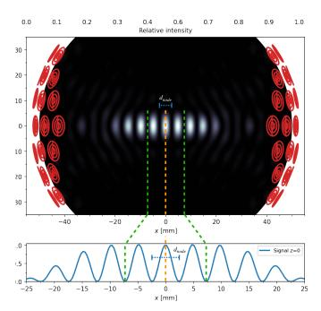
**Figure 4.8:** Simulation of the acoustic trap. The black area shows a simulation of the acoustic field with relative intensity (greyscale) in the region accessible to the CCD. The structures in red color represent the positions and orientations of the transducers. The lower subfigure shows the relative intensity of the acoustic field along the x-axis for the central nodes of the trap.
