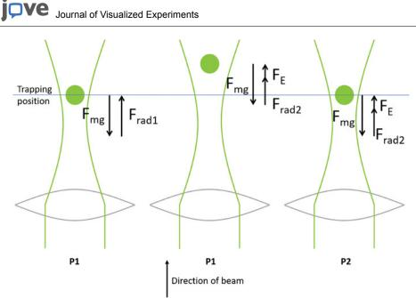
Figure 7: Determination of droplets charge. A schematic sketch of the procedure to determine the absolute charge of an optically levitated droplet. Please click here to view a larger version of this figure.
