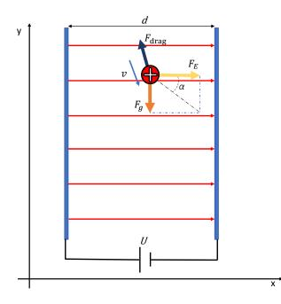
**Figure 3.1:** A small positively charged particle falls into a homogeneous electric field (red arrows).
