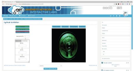
Figure 8: Remote lab interface: trapping a droplet. In remote experimentation, this web application interface is used to trap a droplet. A trapped droplet can be seen in the image provided by the lab webcam due to the scattered light. Please click here to view a larger version of this figure.
