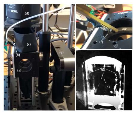
**Figure 4.2:** Left is the experimental setup: (a) experimental chamber, (b) droplet dispenser, (c) turbulence shielding tube, (d) LED-light source, (e) web camera connected to PC. Upper right: (f) close up on droplet charger mounted on the dispenser. Lower right: (g) ITO-plates connected to a voltage supply, (h) falling droplets in curved trajectories due to particle-field interaction (electric force).
