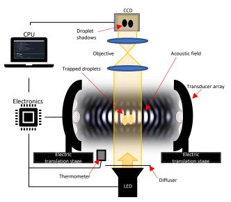
Figure 1. Experimental setup in which the CPU controls the frequency and voltage applied to the transducer arrays of the acoustic levitator. Diffused light from a LED-source passes the acoustic field and is focused on a CCD chip and monitored by the CPU.
