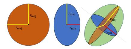
**Figure 3.8:** The oblate spheroid (ellipsoid) to the right is circular (brown, left) when viewed along the dashed axis of symmetry and elliptic (blue, middle) viewed orthogonal to that axis.  $r_{maj}$  is the semi-major axis of the blue ellipse. The semi-minor axis,  $r_{min}$ , in red, of the ellipse is aligned with the axis of symmetry for the oblate spheroid.
