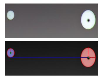
Figure 4. Upper: Image of two levitated droplets. Lower: Extracted pixel-data from upper image. The custom software, finds the regions of white pixels in the upper image and then measures the regions major and minor axis (red lines), as well as the centroid positions (green dot) and the horizontal distance between the centroids (blue line). The red ellipses are painted afterwards using the extracted data, only to show the quality of the elliptic approximation.
