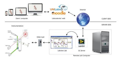
**Figure 5.3:** Remotely controlled experimental setup. "This is adapted from Galán, D., Isaksson, O., Enger, J., Rostedt, M., Johansson, A., Hanstorp, D., de la Torre, L. Safe Experimentation in Optical Levitation of Charged Droplets Using Remote Labs. J. Vis. Exp. (143), e58699, doi:10.3791/58699 (2019)."
