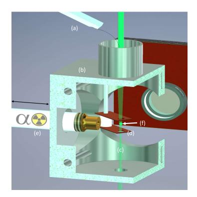
**Figure 4.3:** The experimental setup consists of (a) droplet dispenser and a charger, (b) experimental chamber, (c) a vertical and focused laser, (d) electrodes, (e) alpha source  $(^{241}Am)$  on motorized translation stage, (f) optically levitated droplet. The front and right walls are cut to visualize the center of the experimental chamber.
