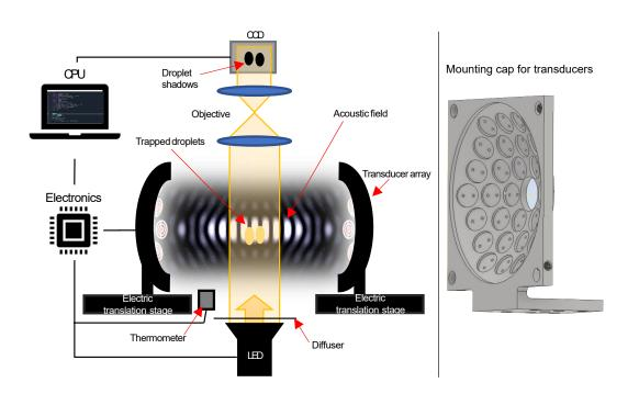
**Figure 4.4:** Left is the experimental setup. The traps acoustic field shown with white antinodes and black nodes. Two droplets (yellow) shadow diffused LED light. The shadows are projected via a camera objective on a CCD chip. The CPU collects the pixel data and the thermometer readings. Right is the design of the mounting cap for the transducers.
