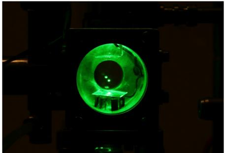
Figure 5: A trapped droplet levitating. In the image it is possible to see one of the droplets levitating inside the cell of the setup. The green color is due to the laser and the fact of seeing two dots instead of one is that the droplet is reflected on the glass of the cell. In this case, the upper point is the reflection and the lower point is the droplet. Please click here to view a larger version of this figure.
