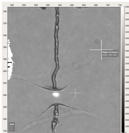
Figure 6.2: A snapshot of an unstable jet exploding as it is hit by X-rays pulses.
