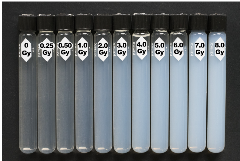
Figure 2: Vials containing NiPAM gel which have been irradiated to different absorbed doses using a dose rate of 600 MU/min.
