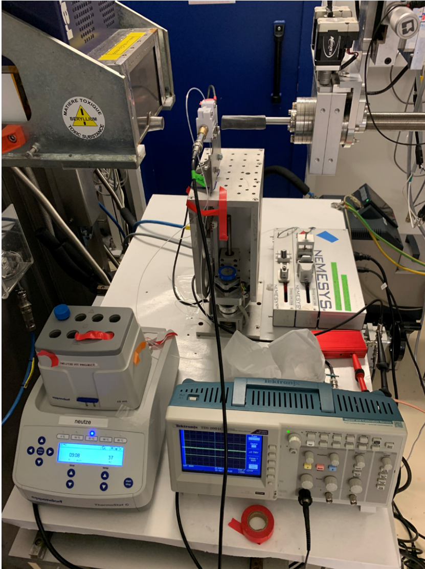
Figure 7.13: Experimental setup for the measurement of potential structural perturbations on microtubules by high voltage alternating electromagnetic fields, ID02 beamline, ESRF
