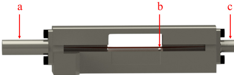
Figure 5.2: Schematic of flowcell. a) 50\ \Omega load, b) hole for imaging. c) connector to coaxial cable.
