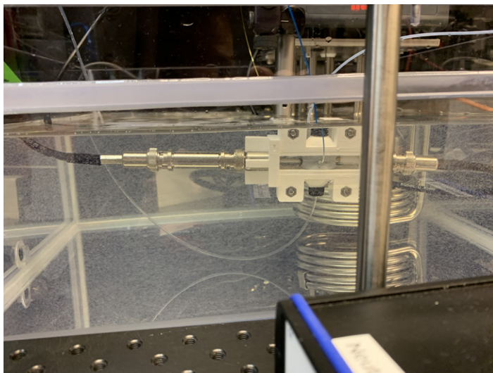
Figure 7.11: Closeup of high voltage flowcell in oil-bath.
