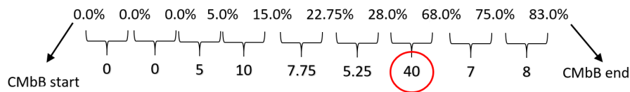
Figure 4.7: The pedal ratio shown in percentages, indicates the pressure by the driver on the accelerator pedal. The numbers on the bottom row show the slope (difference) between two sequential samples. The red circle shows the maximum slope between all the calculated slopes.
