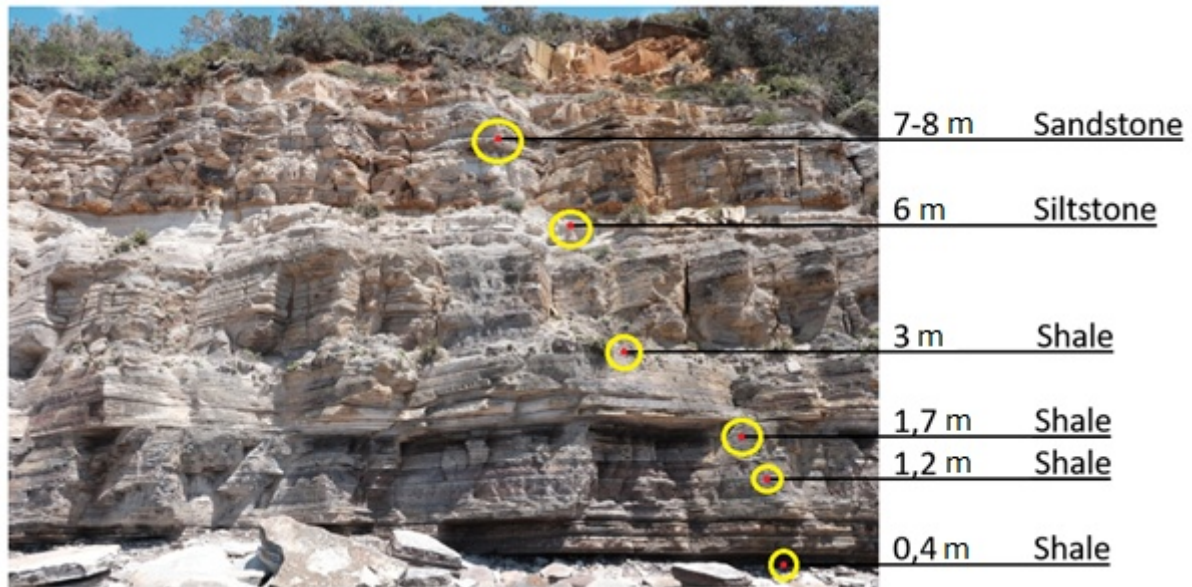
Figure 24. Photograph of the Narrabeen stratigraphy. Edited to show height sequence (m) of where the rock samples were collected from (2018-11-03).
