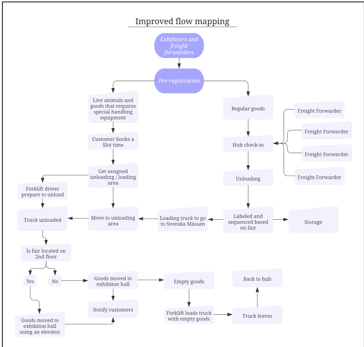
Figure 4: Improved flow mapping of Svenska Mässan's event logistics (Developed by the authors, 2022)
