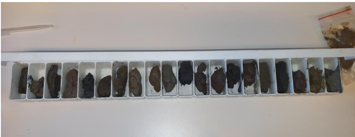
Figure 7. 21 out of the 23 samples that were brought back to the laboratory for further analysis with H 2 O 2 -oxidation.
