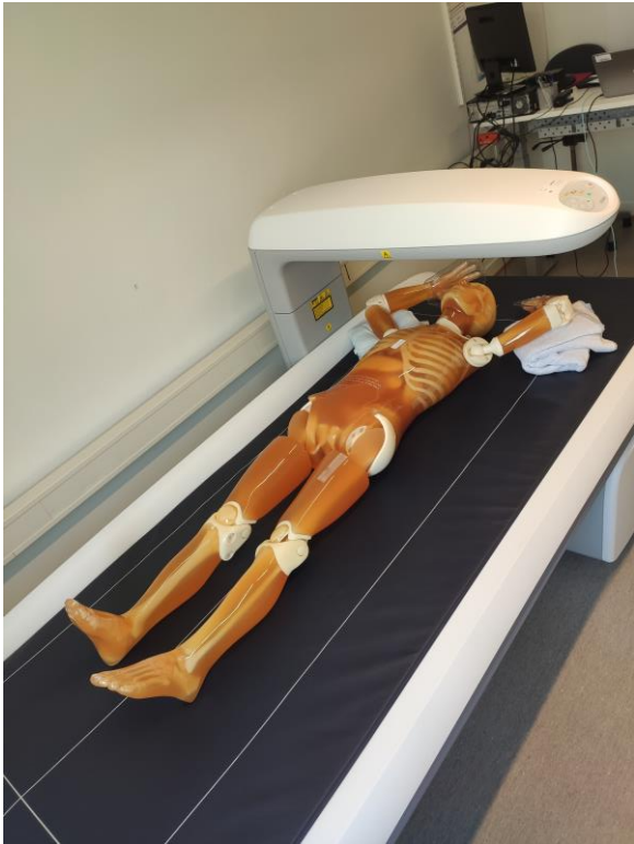
Figure 4: Phantom with BMI 18 (thin) in the GE scanner.
