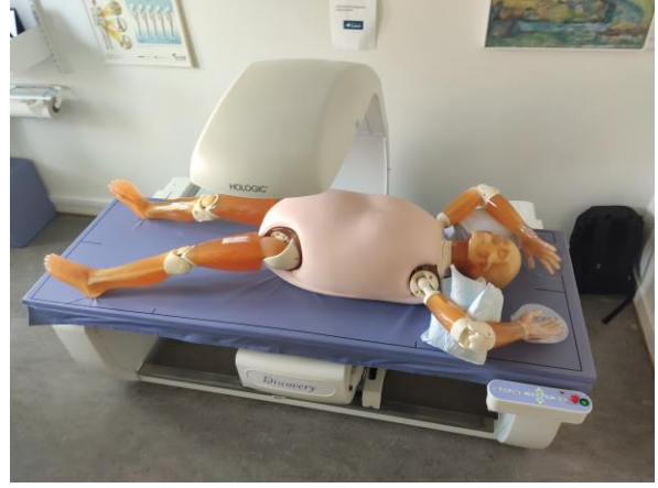
Figure 3: Phantom with BMI 40 (thick) in the Hologic scanner.
