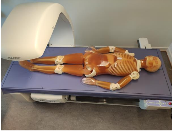
Figure 2: Phantom with BMI 18 (thin) in the Hologic scanner.
