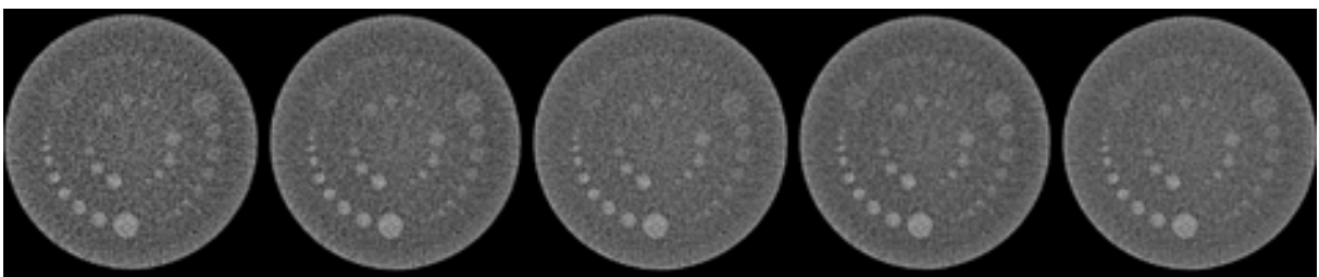
Figure 20: Low contrast for the reconstructions; (left to right) ASIR-V 50%, DLIR-M EC1, DLIR-M EC2, DLIR-H EC1 and DLIR-H EC2, all with NI 3.3
