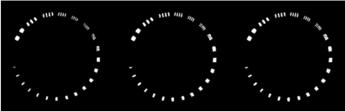
Figure 17: Spatial resolution for the reconstructions; (left to right) ASIR-V 40%, DLIR-M E1 and DLIR-H E1.
