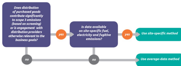
Figure 8: Decision tree for selecting a calculation method for upstream distribution
