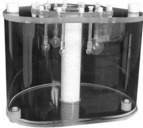
Figure 3: NEMA IQ phantom with a lung insert and six fillable spheres of known internal diameters (35).
