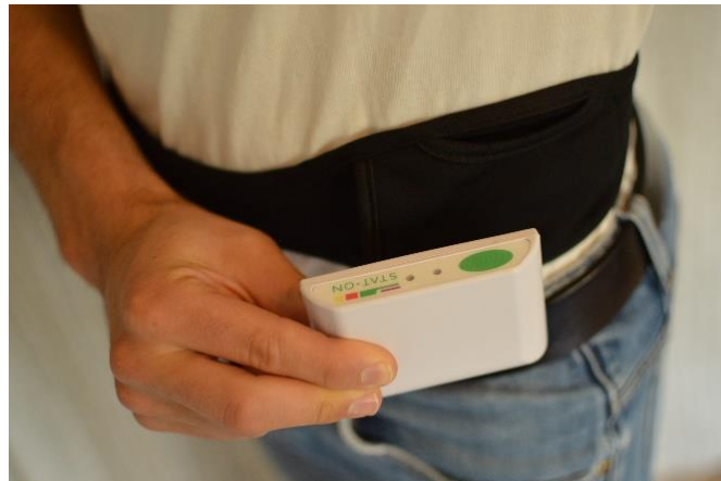
Figure 3. STAT-ON sensor with neoprene belt. (Author's picture)
