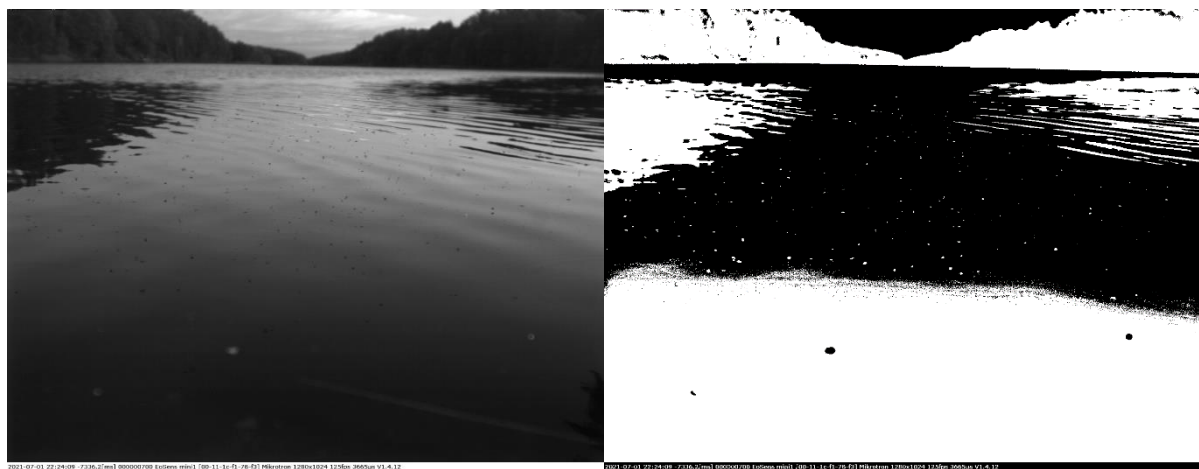
Figure 2 The same frame from a video at lake Långsjön. Left one being the original image and right one after using the Phansalkar local threshold method to create a binary image.
