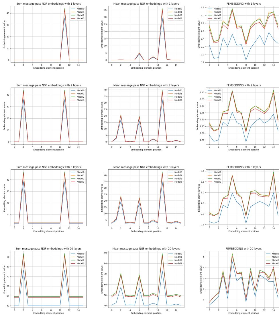
Figure 3.2: Plots of embeddings for the conceptual models. The columns represent the three embedding creation methods that is studied, NGF with sum message pass, NGF with mean message pass and the FEMBEDDING method. The rows show different number of layers included when creating the embeddings, 1, 2, 3, and 20 layers respectively.
