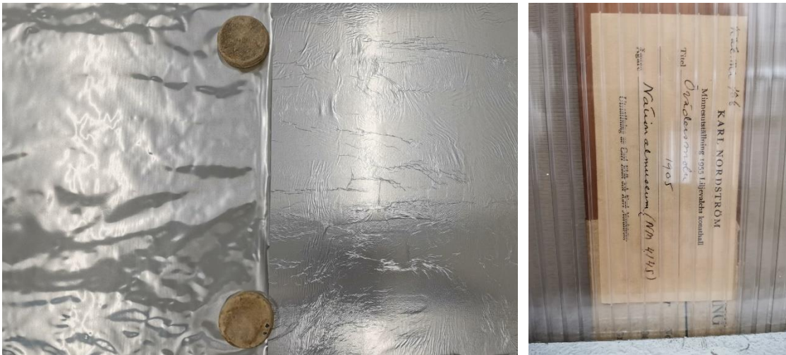
Figure 13:Marvelseal placed on a wooden board to be used as backing for a vitrine (left) and Marvelseal ironed onto the board (right).
