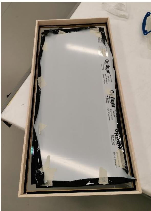
Figure 22: The balsa wood box with glazing and protective plastic. The box is a separate unit that can be lifted out of the frame.
