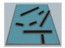
Figure 2.13: Visualization of a navmesh in a small environment where the gray is the environment, the black objects are impassable walls, and the blue layer atop the environment is the navmesh  $^{5}$ .
