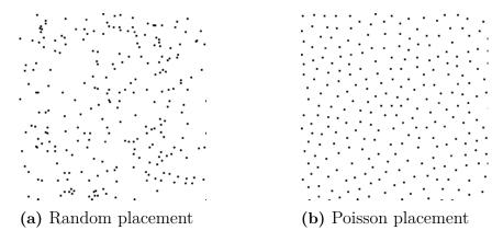
Figure 2.11: Example of two point generation methods<sup>3</sup>. Selecting points with completely random coordinates results in some clustering and some clear parts of the field, as can be seen in 2.11a. The method presented in figure 2.11b visualizes points generated with an algorithm used to create a *Poisson Disk Sample Set* [23].
