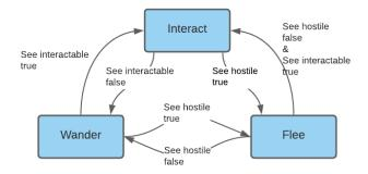
Figure 2.2: FSM example: the nodes correspond to states, edges are transitions and weights are conditions. Inspired by: [11, Chap. 9].
