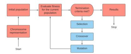
Figure 2.4: A flowchart diagram representation of a GA. Each container represents a step in the algorithmic sequence, ranging from chromosome representation, evaluating fitness function and checking for termination criteria. Until termination criteria is met, iterations of selection, crossover and mutation is processed between the fitness evaluation step to improve the solution.
