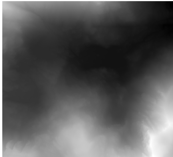
Figure 2.2: 1m resolution elevation raster for a 5\text{km}^2 area. Lighter pixels correspond to a higher elevation value.
