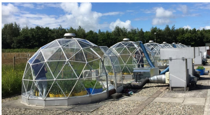
Figure 3. Solar domes used to control levels of O 3 and temperature at the UK Centre for Ecology & Hydrology air pollution exposure facility in Abergwyngregyn (Wales). Photo by Malin Broberg.
