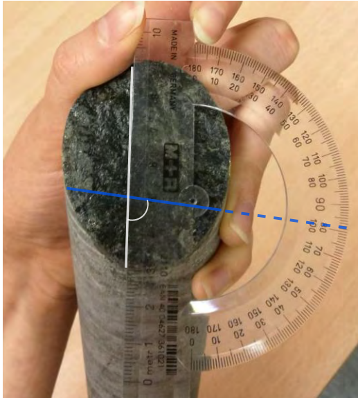
Figure 8. Blue line showing the lineation and white line showing the fracture plane. Protractor used to determine the pitch.
