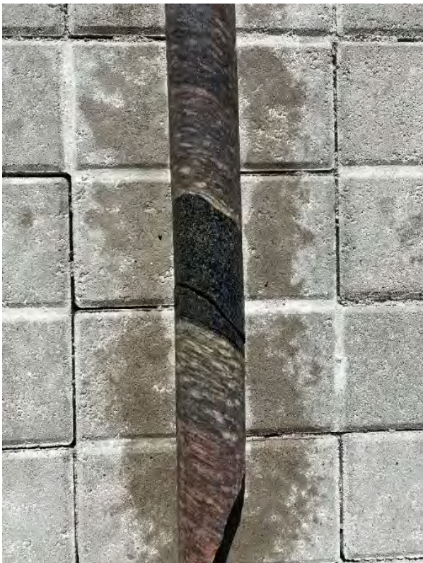
Figure 22. Biotite zone with mylonitic texture at 319,65m depth of the GE1 drill core.
