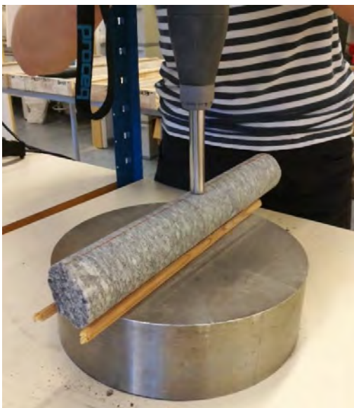
Figure 9. Setup for the Schmidt hammer test, two wooden strips attached to a 30 kg steel base.
