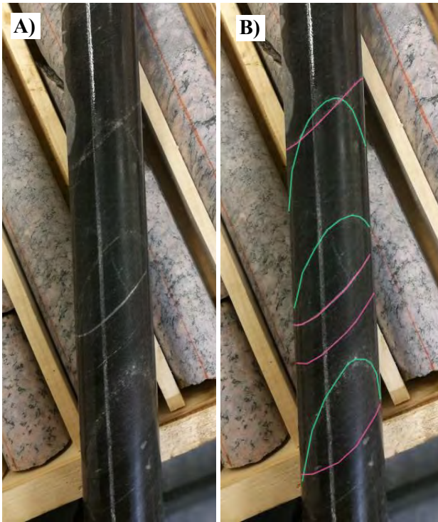
Figure 21. A) Overprinting foliation at depth 126,2m of the GE1 drill core. B) Highlighted overprinting foliation at corresponding depth, where green is the older foliation and pink is the overprinting.
