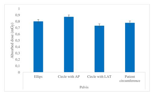
Figure 18. The estimated fetal absorbed doses for the patients using either the more exact patient circumference or approximating the circumference to an ellipse or circle for the CODE method in the pelvis protocols. The error bar shows the standard error.
