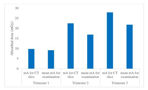
Figure 16. The fetal absorbed dose for the phantom for the different trimesters when using either the specific CT slice tube current or the mean tube current for the examination in CT-Expo. The error bar shows the standard error.
