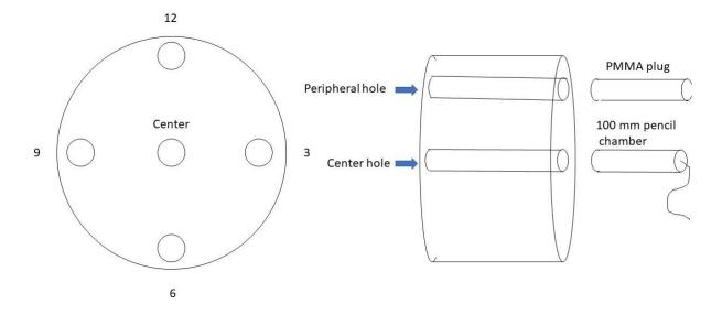
Figure 3. The general set up for the CTDI<sub>100</sub> measurement in a standard CTDI PMMA phantom. There are two standard CTDI phantoms, 16 cm or 32 cm in diameter representing head or body respectively, both are 15 cm in length. The pencil chamber is 100 mm long and is placed either at the centre or at the periphery holes of the phantom. Unused holes may be plugged with PMMA rods. This picture is modified from an illustration in AAPM 204 (AAPM204, 2011).
