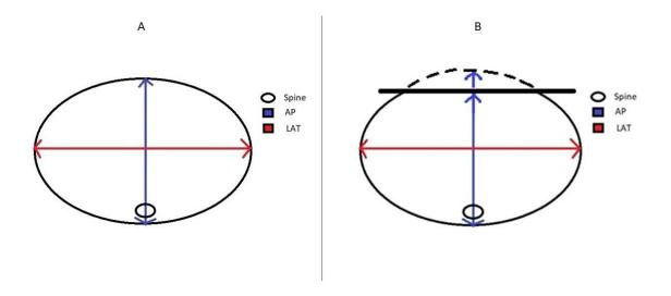
Figure 4. A) shows the AP and LAT dimensions in an axial CT slice with the spine as a reference. B) Shows an example if the AP dimension was cut off where the long blue arrow represents the visible part of the AP dimension. The dotted line represents the approximate size of the patient outside the dFOV and the long + short blue arrow represents the approximate AP dimension. If the LAT dimension was cut off the same method was applied there.
