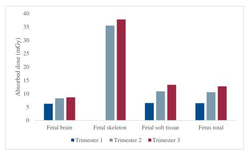
Figure 23. The absorbed doses to different organs of the fetus and the total dose to the fetus for the phantom estimated by VirtualDoseCT for the phantom measurements using an abdomen protocol.
