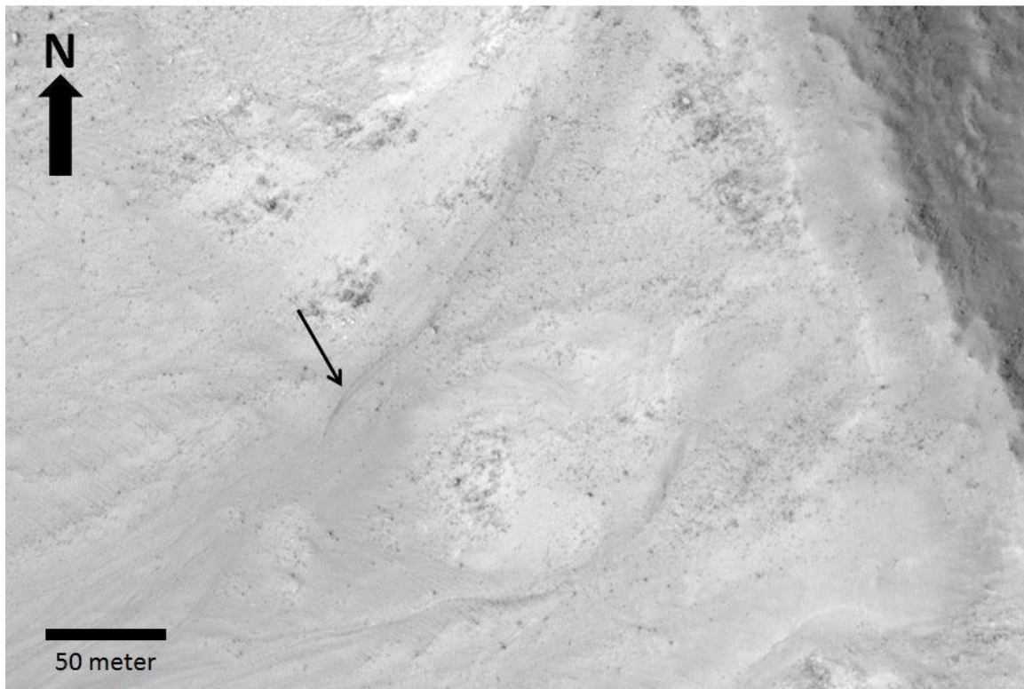
Appendix Figure 3: Hiview image of NE part of crater in ESP_034909_2300. The slope direction is SW. Solar incidence angle 43^\circ , with the Sun about 47^\circ above the horizon. Arrows in image point to potential RSL's. Credit: NASA/JPL/University of Arizona.
