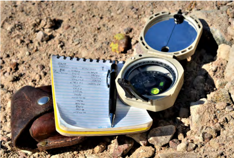
Figure 3.2: Typical tools used for fabric measurements, a Brunton compass, notebook, and pencil. Photo: Gustaf Peterson Becher.
