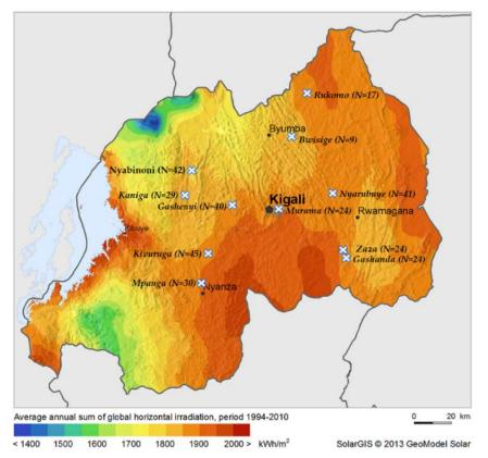
Figure 1. Sectors Surveyed and Global Horizontal Irradiation Levels
