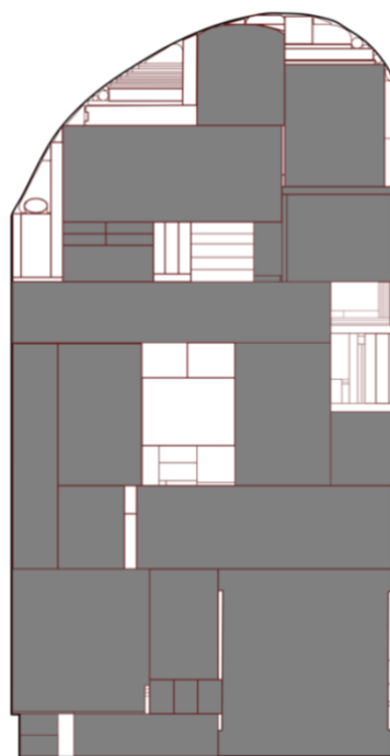
Figure 8: Illustration of the structural base on side B. Each object is outlined, and the objects that creates the structural base are filled in
