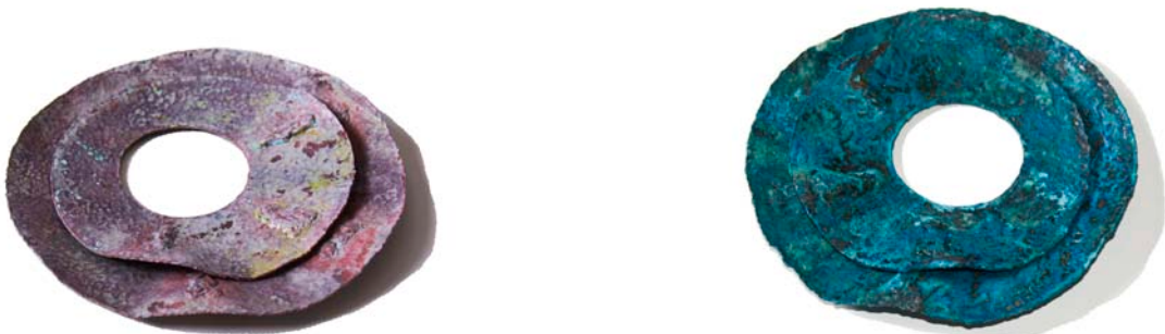
Fig. 36 a, b. These pictures display some experimental patinated copper samples, recently realized. Silvia Corti, 2020.
