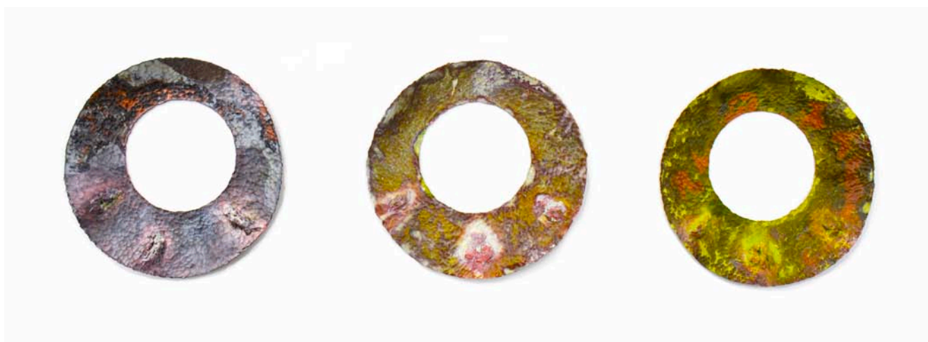
Fig. 16. Some copper samples treated with the same mixture but exposed respectively: one hour, one day and one week. Silvia Corti, 2020.
