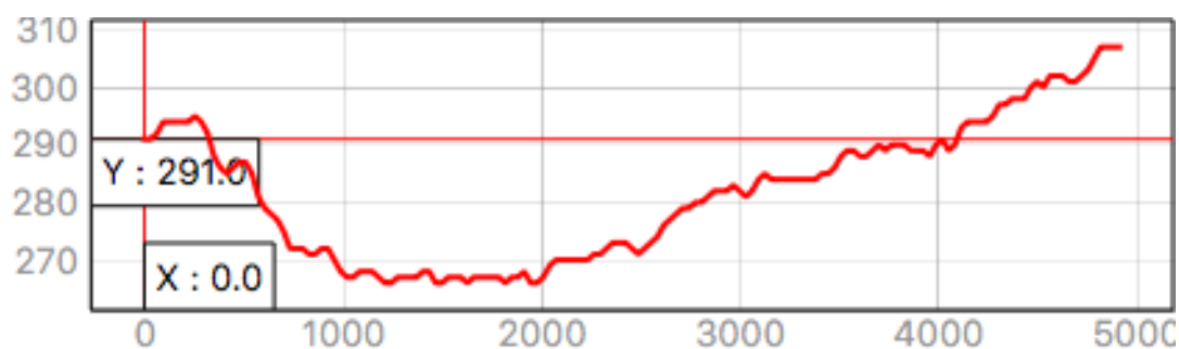
Figure 14: A transverse cross section of Wadi D. The length of the cross section is ~4,9 km and the vertical axis shows a height difference of ~27 m between the level of the wadi and the uplands. Vertical exaggeration is about x30. Location of the cross section is seen in figure 10.
