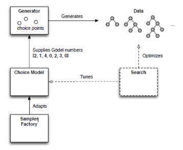
Figure 2.1: GödelTest Framework Architecture [5]
