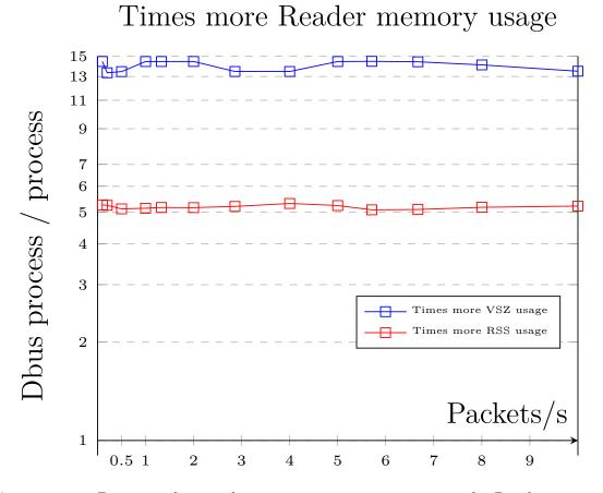
Figure 4.12: Diagram showing how many times more memory the Reader process uses when D-Bus is included.
