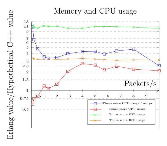
Figure 4.16: Diagram showing how many times more memory and CPU the Erlang prototype require compared to a hypothetical C++ prototype.
