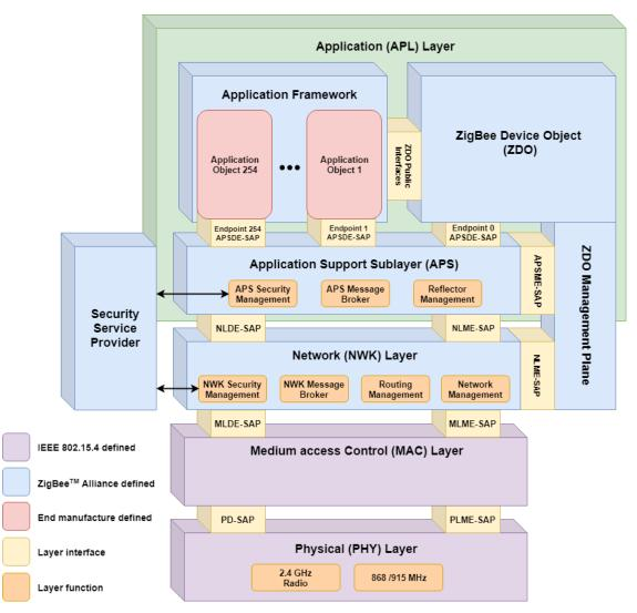
**Figure 2.5:** Image of the ZigBee stack architecture based on ideas from Gislason (2008); Yang (2014); ZigBee Alliance (2012).
