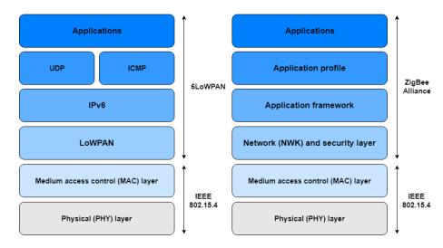
Figure 2.2: 6LoWPAN stack and ZigBee stack on top of the IEEE 802.15.4 stack
