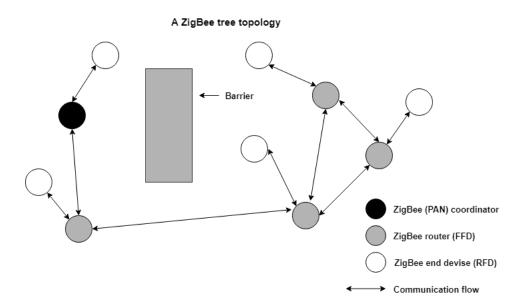
Figure 2.4: A ZigBee network topology with a barrier.
