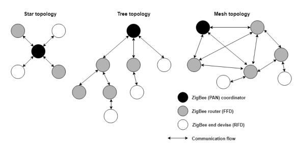
Figure 2.3: ZigBee network topologies
