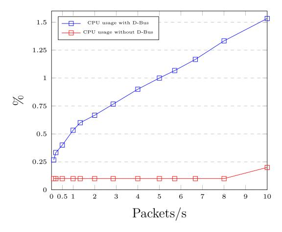
Figure 4.13: Data about the CPU usage of the Reader process collected from the ps command.
