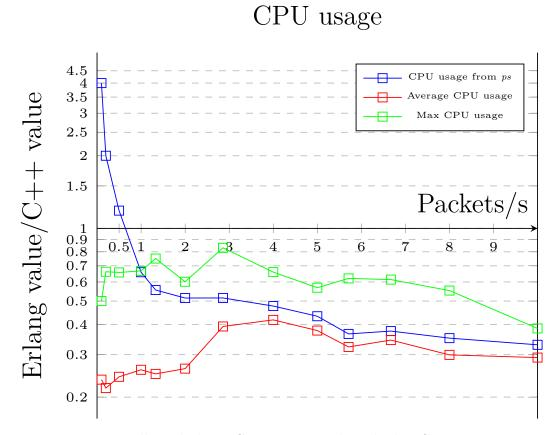
Figure 4.7: Data collected about CPU usage as described in Section 3.3.
