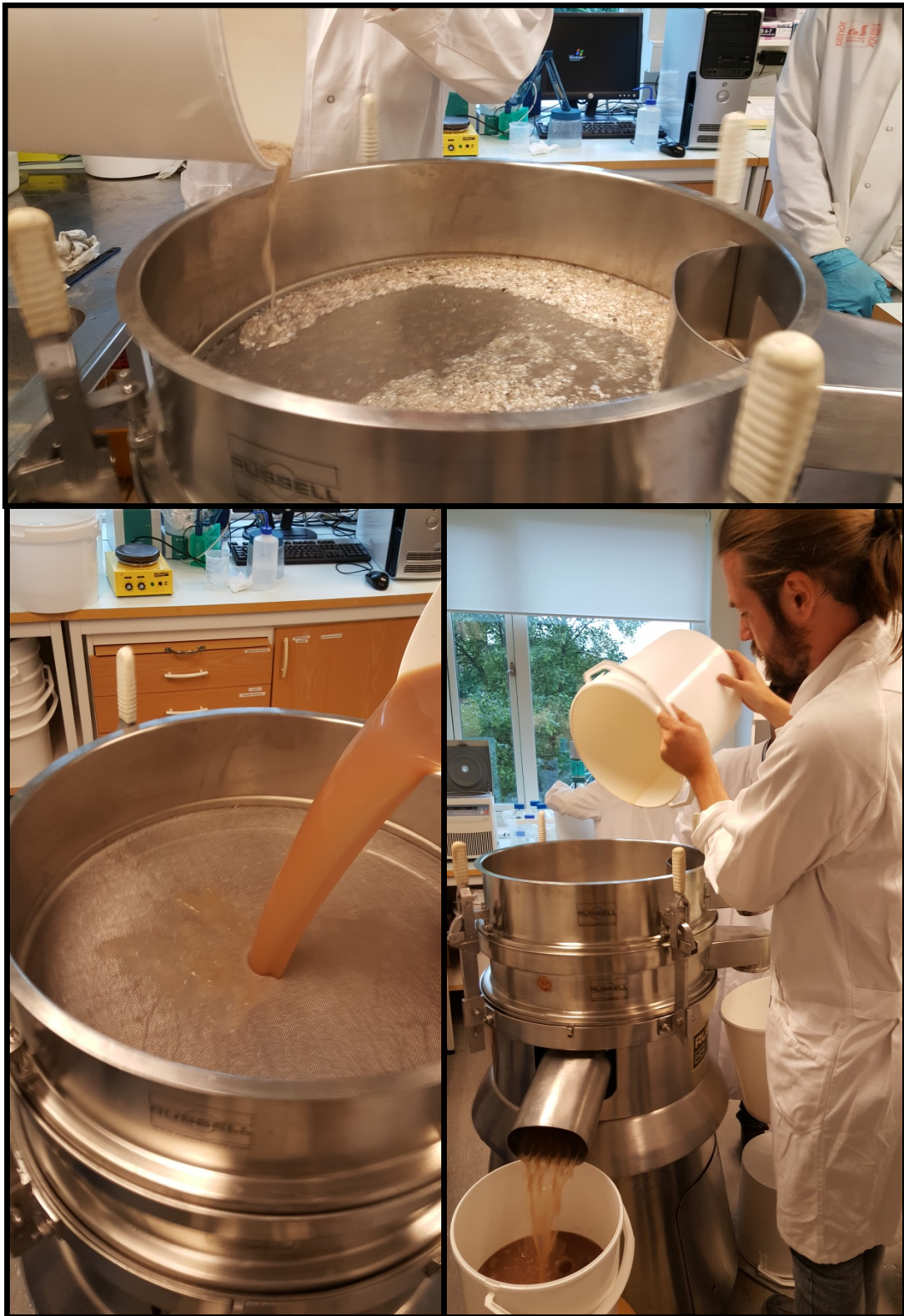
Figure 11: Large-scale application of the pH shift process using commercial sieve technology. Instead of using gravity as the separation step (as done in paper I), a filter with mesh size 10 \mu\text{m} was used to separate different fractions in step 1 and step 2 of the pH shift process.
