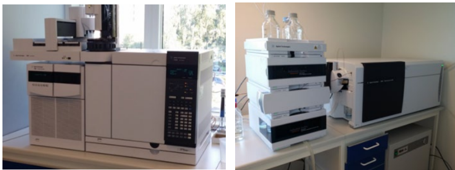
Figure 8. Equipment for gas chromatography–tandem mass spectrometry (left) and liquid chromatography–tandem mass spectrometry (right).
