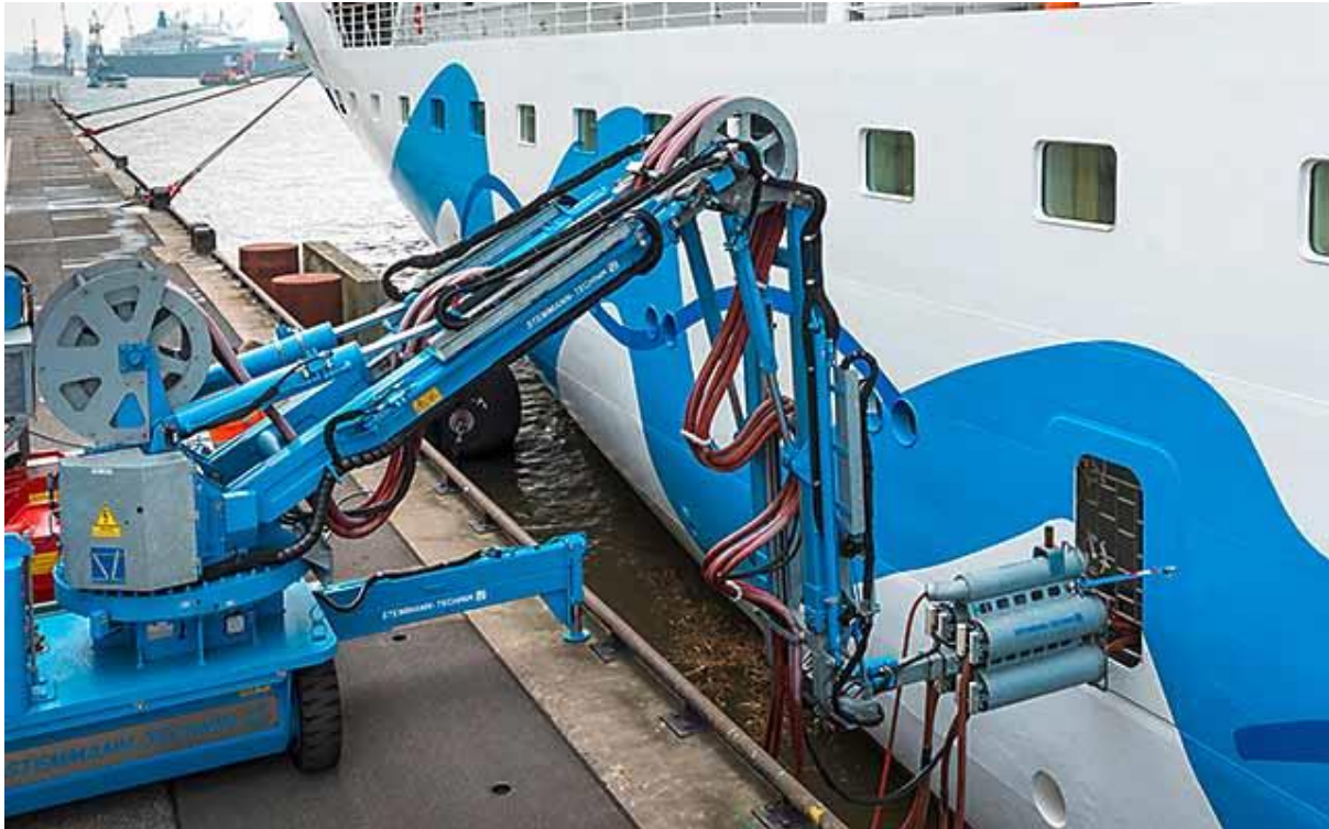
Figure 2: Onshore Power Supply (OPS). Source: DNVGL, 2018
