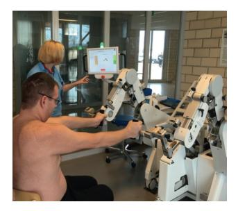
Figure 10. MotionMaker TM in the mode to measure the pushing force of the arms
