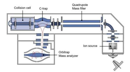
Figure 9. Schematic representation of a Q-Exactive instrument (courtesy of Thermo Fisher  $\mbox{\ensuremath{\mathbb{B}}}\xspace$
