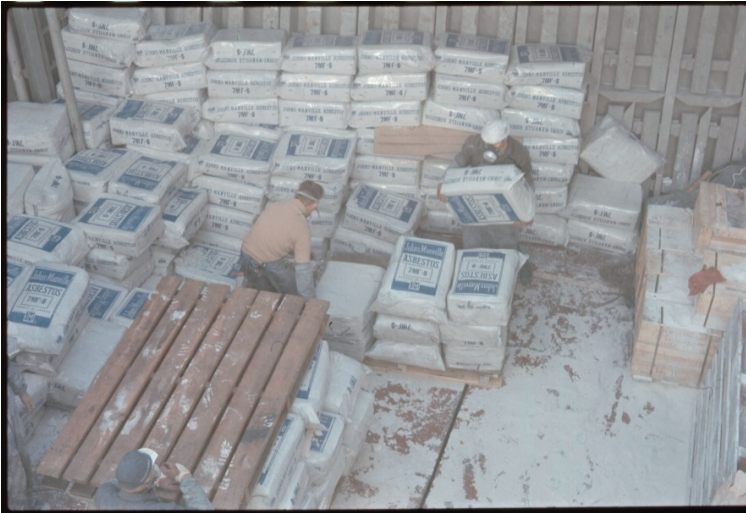
Figure 1. Stevedores in Gothenburg harbour unloading packages of asbestos in the 1970'ies. The workers only use a protective mask for dust. With permission from the Port of Gothenburg (Göteborgs Hamn AB).
