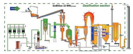
**Figure 16.** A schematic of the GoBiGas gasification section. 1, gasifier; 2, combustion chamber; 3, cyclone; 4, post-combustion chamber; 5, raw gas cooler; 6, raw gas filter; 7, rapeseed methyl ester scrubber; 8, carbon beds; 9, flue gas train; 10, fuel feeding system. (Illustration from Göteborg Energi AB).
