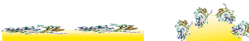
Figure 5.3.1 Illustration of how high curvature support enables retained enzyme tertiary structure upon immobilization.
