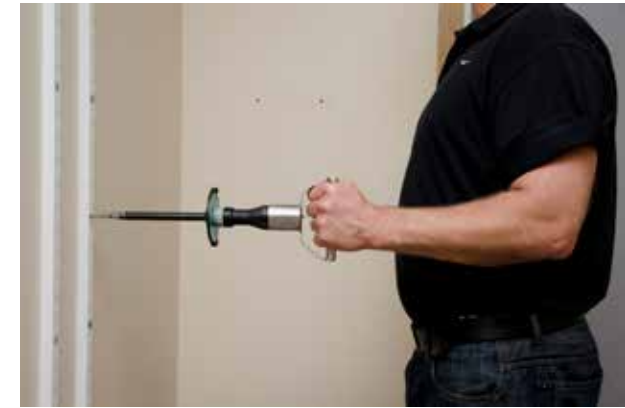
Figure 22. Torque measurement using the Tohnichi screwdriver.
