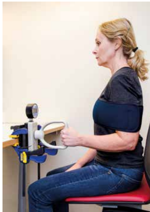
Figure 34. Torque strength measurement, seated position.
