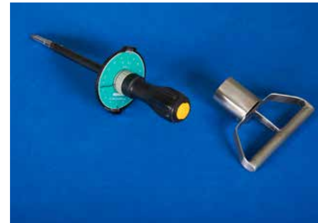
Figure 23. Tohnichi torque screwdriver with custom-made handle.
