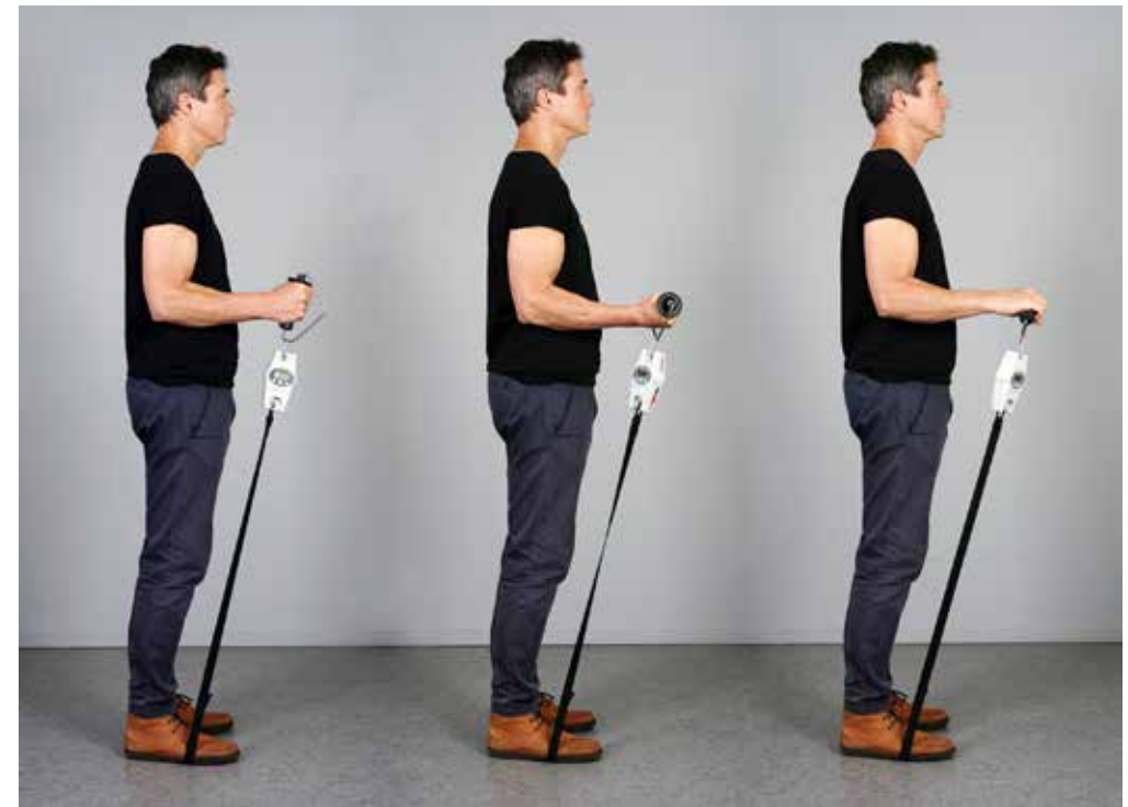
Figure 15. Lifting strength measurement using Kern dynamometer. Neutral, supinated and pronated position ©.
