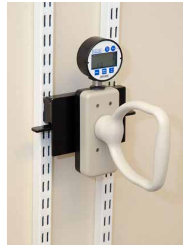
Figure 25. Baseline dynamometer with shovel handle, wall-mounted on rails.
