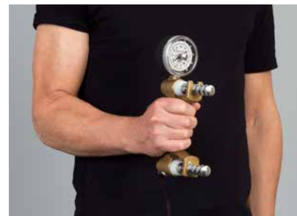
Figure 13. Grip strength testing with the Jamar dynamometer ©.
