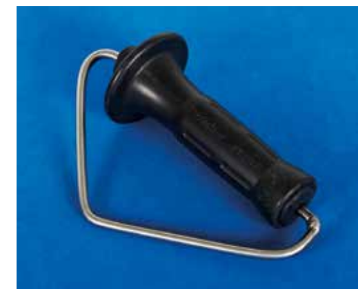
Figure 20. Custom-made handle used with the kern dynamometer.
