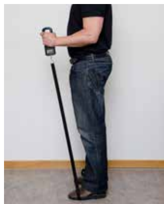
Figure 18. Lifting strength measurement using Daiwa Mission dynamometer.
