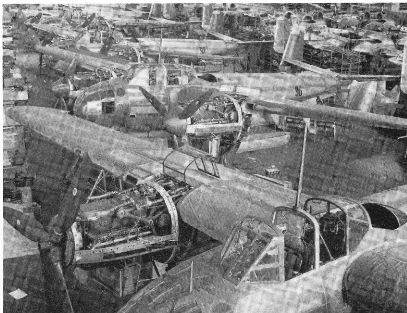
SAAB 18 Bs under construction in Linköping. The engines are DB 605s which differ greatly from those previously manufactured in Sweden. Inter alia they had hanging cylinder blocks with 12 cylinders forming a V and a fuel injection pump (Övl. Kindberg, Flygstaben).
