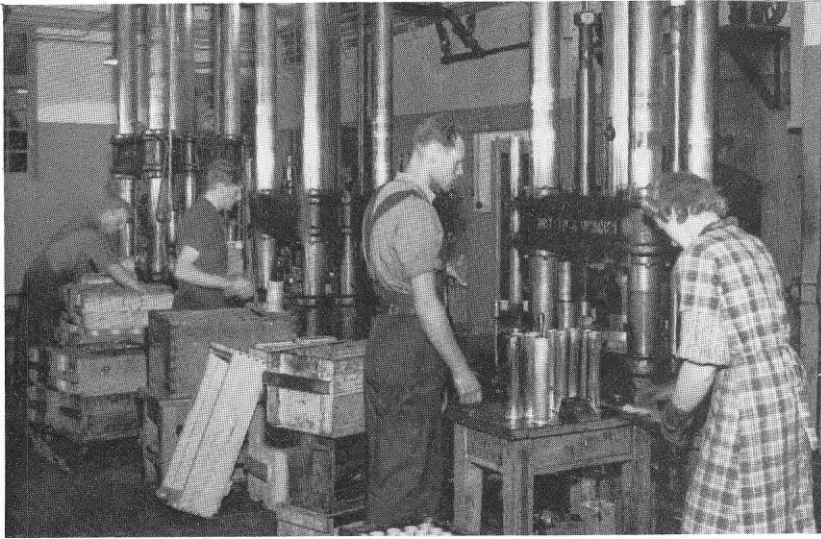
The throttling and drawing of cartridge cases at the ammunition factory in Marieberg in June 1940 (Fst pressdetalj).
